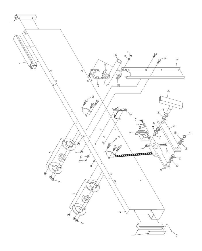
Right Drive Frame Assembly (Machine Series 443 and Above)
