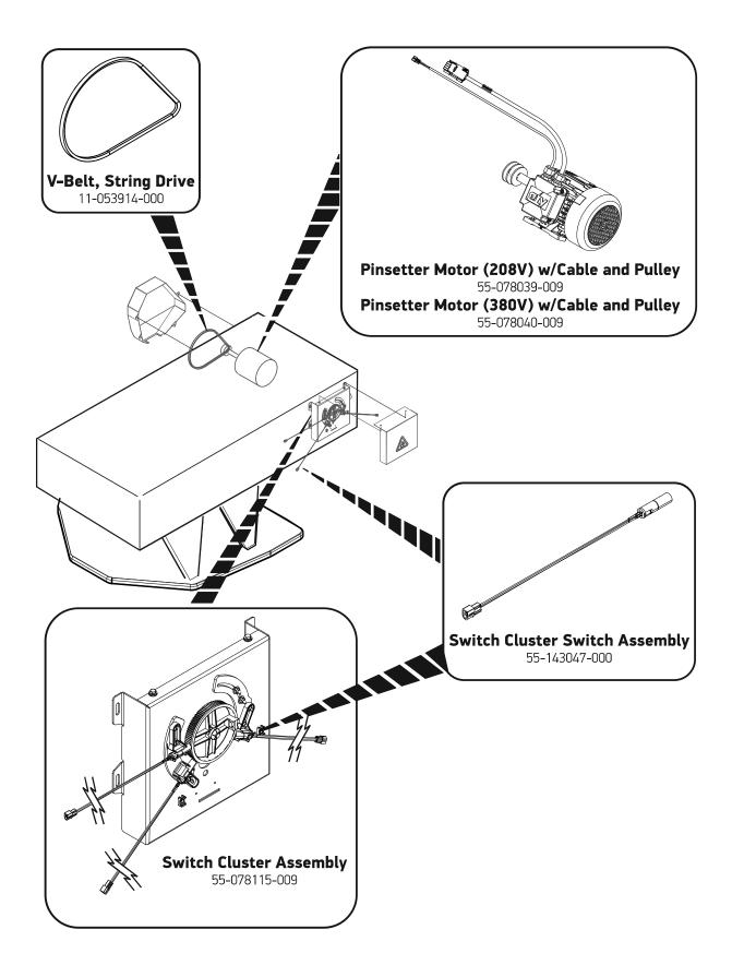
Pinsetter Motor / Switch Cluster Assemblies
