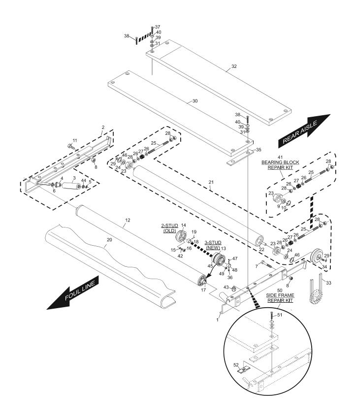
Transport Band Assembly (10 mm Side Frames) Short Pit Machines Series 208 and Above
