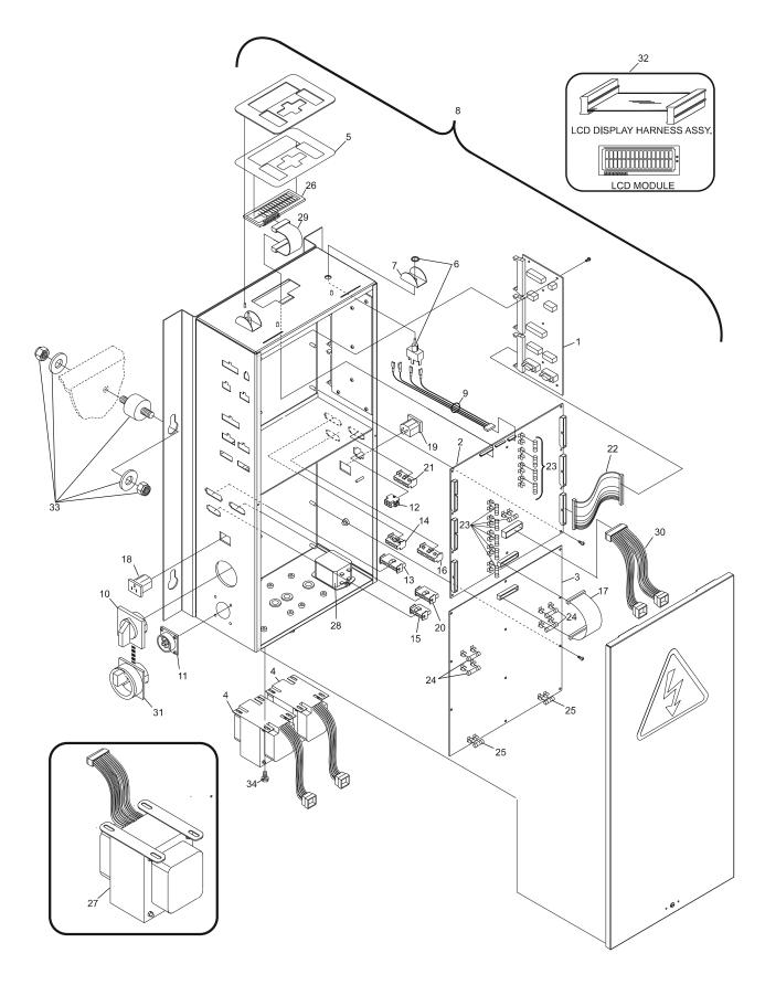
Nexgen Controller Assembly (Includes Internal Cabling)
