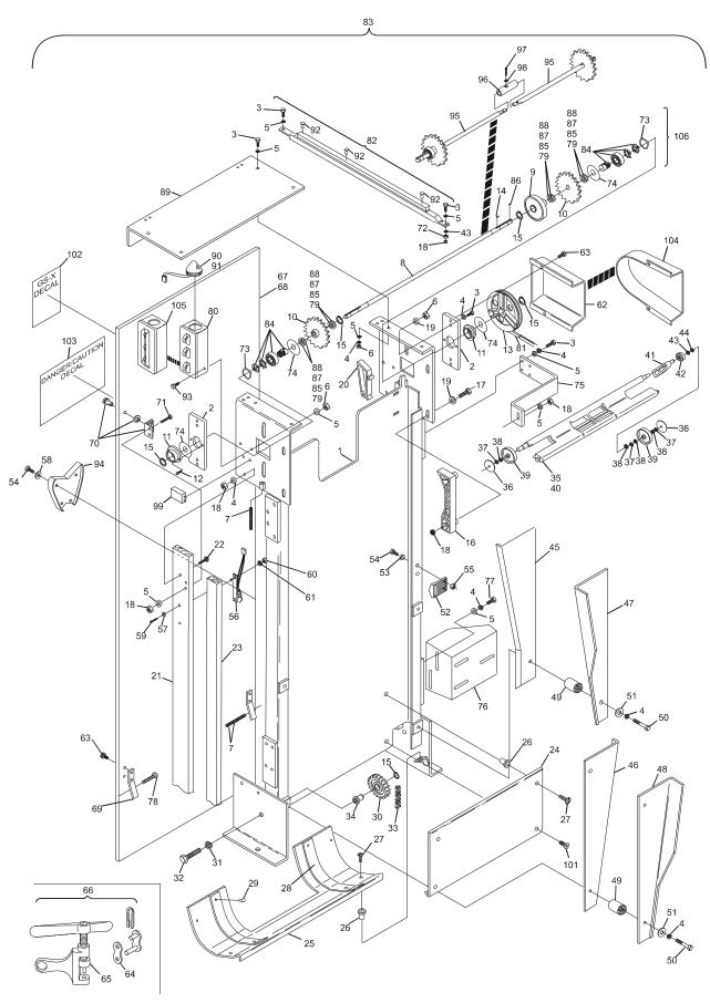
**Elevator Assembly - Square Frame Hole Short Pit Machines Series 43 and Above**
