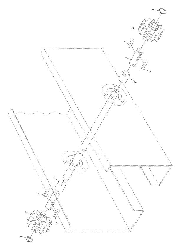
**Setting Table Pinion Shaft Assembly**
