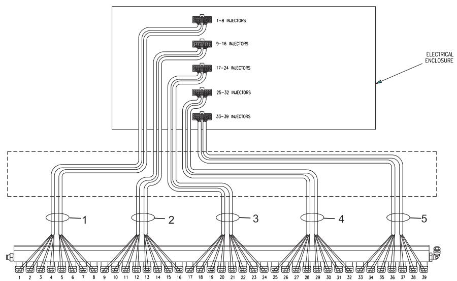
**Electronic Enclosure - Rear View - Cable Assemblies**
