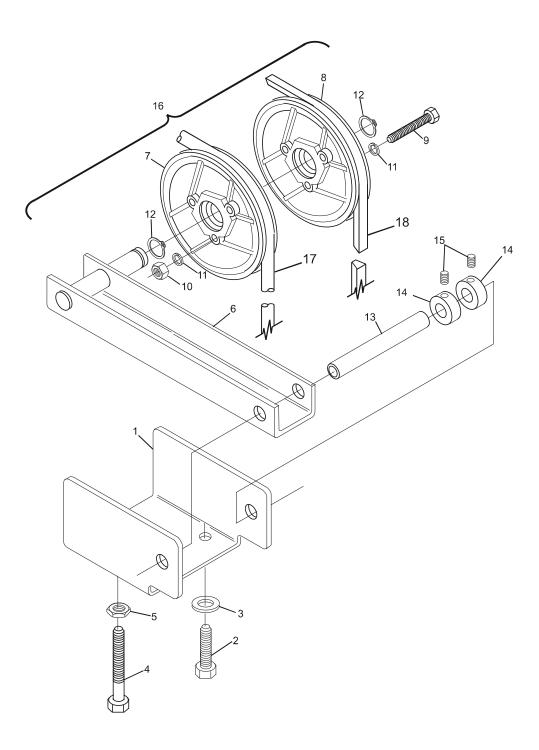
Transport Band Belt Tensioner Assembly - Right Machine Short Pit Machines Series 43 and Above
